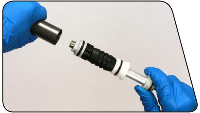
**4** Spray isopropyl alcohol on the inside and outside of the air tube and wipe it with a clean rag. Wrap a clean rag around a long dowel and insert it into the air tube to clean inside the air tube.
