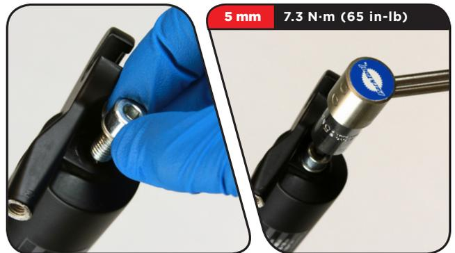
**8** Insert the external rebound damper knob into the rebound damper shaft bolt until it is secure. Adjust rebound as desired.
