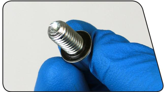
**7** Insert the shaft bolts into the threaded shaft ends through the shaft bolt holes. Use a torque wrench with a 5 mm hex bit socket to tighten the bolts to 7.3 N·m (65 in-lb).
