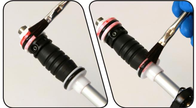
**11** Firmly push the air assembly into the bottom of the upper tube while gently rocking the air shaft side to side.
