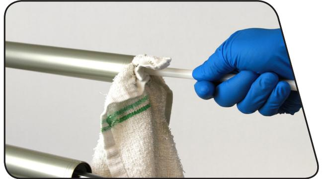
**5** Slide the base plate/negative piston assembly, top out bumper, and travel spacer (if applicable) from the air shaft. Spray the air shaft with isopropyl alcohol and wipe it clean with a rag.
