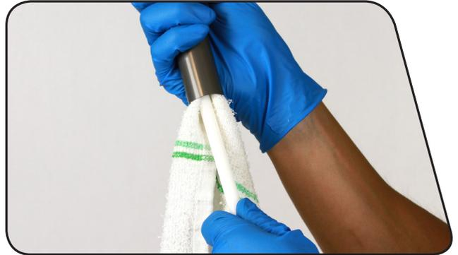
**5** Slide the negative piston assembly from the air shaft. Spray the air shaft with isopropyl alcohol and wipe it with a clean rag.
