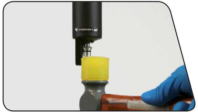
**6** Firmly pull the lower leg downward until oil begins to drain. *If the upper tubes do not slide out of the lower leg or if oil doesn't drain from either side, the press fit of the shaft(s) to the lower leg may still be engaged. Reinstall the shaft bolt(s) 2 to 3 turns and repeat the previous step.*
