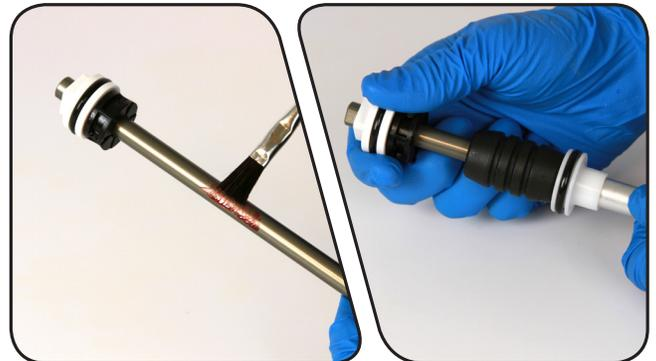
**9** Apply grease to the inside of the upper tube, from the end of the tube (opposite the crown) to approximately 60 mm into the tube.
