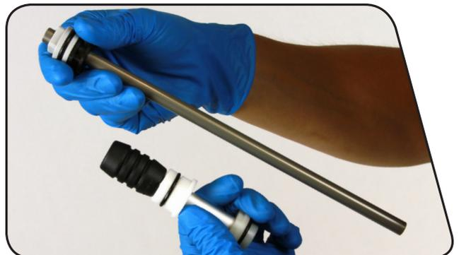
**6** Use a pick to remove the air piston outer o-ring. Apply grease to the new o-ring and install it.
