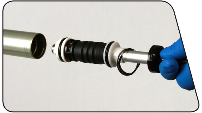
**4** Spray isopropyl alcohol on the inside and outside of the upper tube. Wipe the outside of the upper tube with a clean rag. Wrap a clean rag around a long dowel and insert it into the upper tube to clean inside the upper tube.
