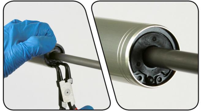
**12** Use a pick to remove the top cap o-ring. Apply a small amount of grease to a new top cap o-ring and install it. Apply a small amount of grease to the top cap threads.
