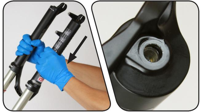
**6** Clean the shaft bolts, crush washers, and crush washer retainers. Inspect the crush washers and retainers. If the crush washers or retainers are flattened or deformed, replace them with new ones.
