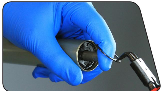
**3** Firmly pull on the air shaft to remove the air spring assembly from the upper tube. Clean and inspect the assembly for damage.
