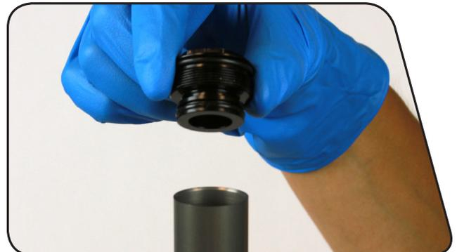
**3** Remove the air shaft/piston assembly from the bottom of the air tube by pulling the shaft down and rocking it from side to side.
