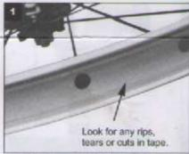
Inspect clear amber colored tape to make sure it will hold air and seal against the tire bead.
