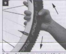
Once the beads are seated and the tire is holding air with seatant inside, you will need to shake the wheel evenly to spread the seatant in the tire until any small air leaks are seated. Shake in many directions.
